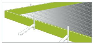
Engineered LVL edge boards are used in formwork applications
