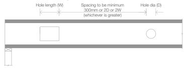
\*Minimum spacing between holes must be at least 300mm or twice the diameter or length of the largest opening (whichever is greater)
