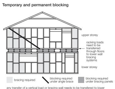
any transfer of a vertical load or bracing wall needs to be transfered to lowe storey walls to enable the loads to flow through to the building foundations
