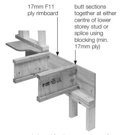
note: use rimboard for the upper storey of two storey construction or the sub-floor for single storey construction
