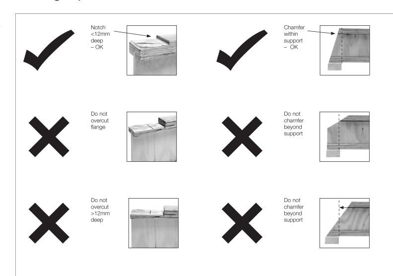
Seek technical advice before chamfering the joists beyond the bearing supports as plywood reinforcing may be required.
