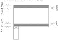
\*Flanges can be notched at supports as per installation guide, but no cuts on or within 5mm of the flange are allowed
