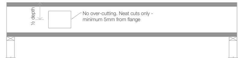
\*Holes recommended to be mid height of joist
