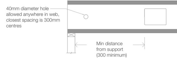
\*Refer to service hole guide for minimum distance from supports
