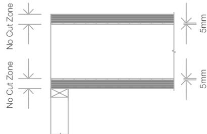
\*Flanges can be notched at supports as per installation guide, but no cuts on or within 5mm of the flange are allowed
