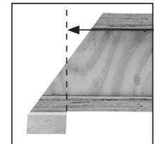
Seek technical advice before chamfering the joists beyond the bearing supports as plywood reinforcing may be required.
