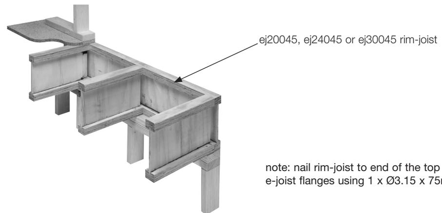
note: nail rim-joint to end of the top and bottom e-joint flanges using 1 x Ø3.15 x 75mm nail
