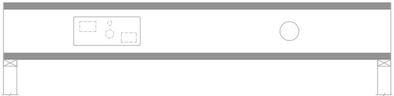
\*Smaller holes can be grouped into a larger hole subject to the maximum size being within the service hole guide limits
