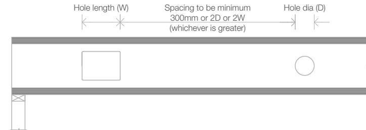
\*Minimum spacing between holes must be at least 300mm or twice the diameter or length of the largest opening (whichever is greater)
