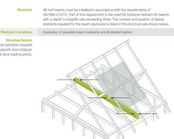
Beam lateral restraints required at supports and midspan (at the strut loading point).
