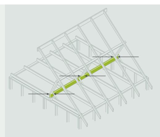
**Strutting-Hanging Beams** Beam lateral restraints required at supports and midspan (at the strut loading point).
