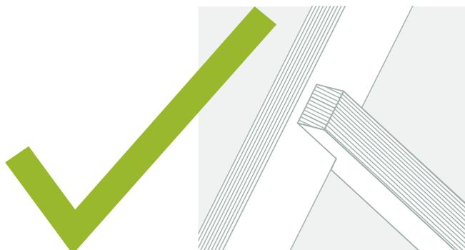
Fix the bottom of the e-strut to the support with 2 x 3.15mm $\varnothing$  framing nails driven through the face of the e-strut.
