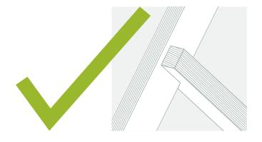
Fix the bottom of the e-strut to the support with 2 x 3.15mmø framing nails driven through the face of the e-strut.
